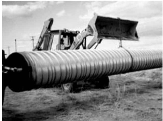
ULTRA FLO is available in long lengths. And, its light weight allows it to be unloaded and handled with small equipment.
