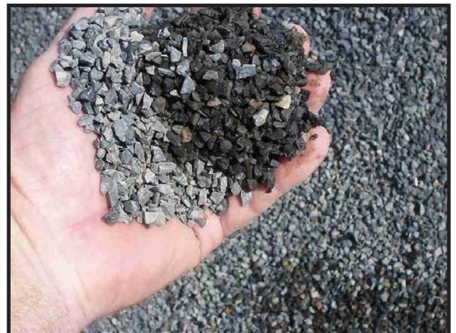
Sample of crushed aggregate for use in concrete.
