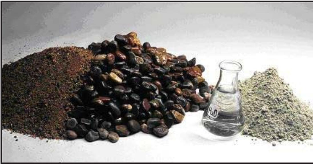
From left to right: fine aggregate (sand), coarse aggregate, water, and cement.
