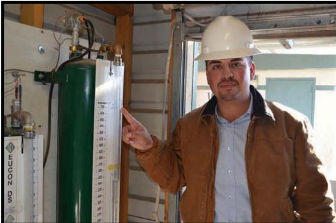
Daniel Quezada points out the equipment used to measure the amount of admixture that will be added to the concrete.
