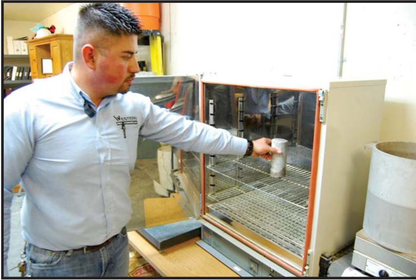
Daniel Quezada prepares a core sample for absorption testing.
