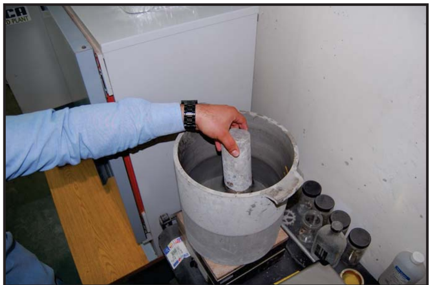
Example of core sample immersed in water after drying to test absorption.
