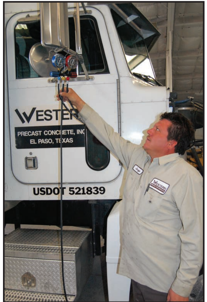
Jorge Olmos sets up cooling gauges for preventive maintenance.
