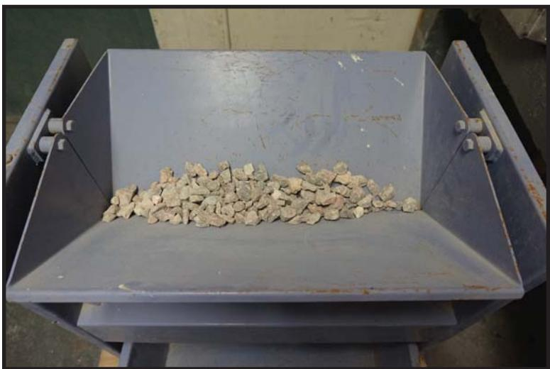
**Aggregate sample is divided into smaller portions using an aggregate sample splitter.**
