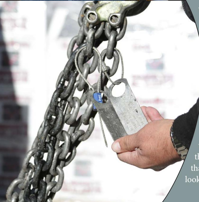
As the close to 2016 approached, Western Precasts' hardworking employees finalized inspections for the year. We focused on the entire rigging setup to include tie down straps, cables, blocks and hooks. I personally looked for cuts on straps, nicks and abrasions on our chains and made certain that the sure-lock hooks were working properly.
