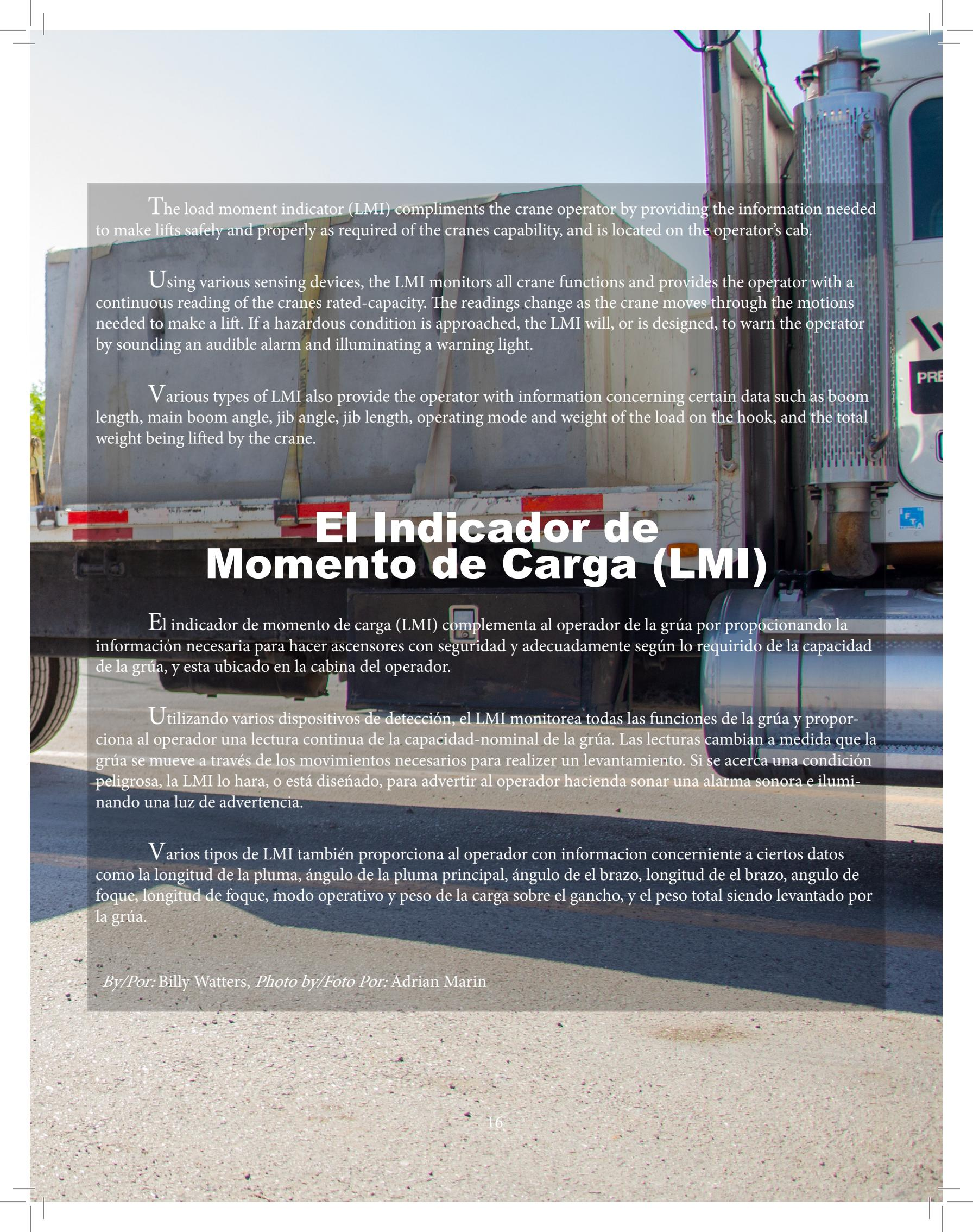
The load moment indicator (LMI) compliments the crane operator by providing the information needed to make lifts safely and properly as required of the cranes capability, and is located on the operator's cab.
