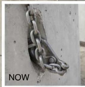
The production department is always looking for ways to improve our production practices to enhance our efficiency and safety guidelines. One of the practices that we have improved greatly over the years is the use of rigging devices and embedded anchors for handling the concrete structures that we manufacture.
